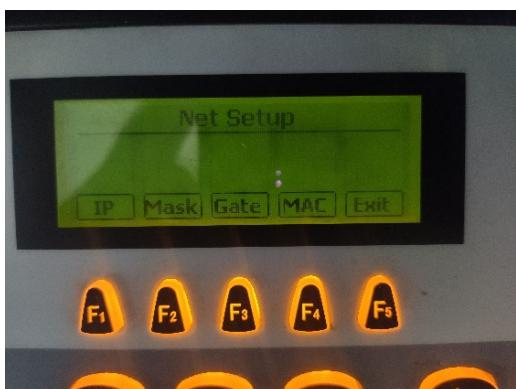
(2) Press the corresponding soft key into modify interface, and press number key to change the value of cursor position. Press 【PREV】key to move the focus forward, press 【NEXT】、【ENTER】 keys to move the focus back. Press <Exit> key to return the previous menu.
