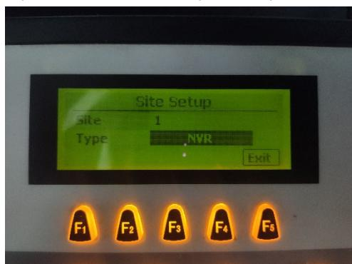
Press 【PREV】、【NEXT】 key in the type selection input box to select to control device, press 【ENTER】 to confirm, and into corresponding device property setting interface.
