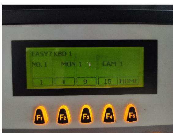
(4) Press 【Shift】+【Site】 , and input the IP address of PC which Easy7 is installed on. After setting, Press 【Shift】+【Site】 to exit setting.
