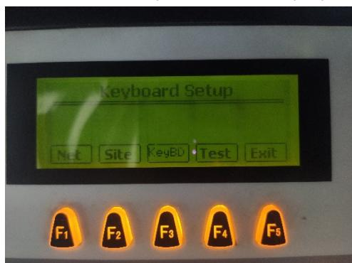
(2) Every keyboard support to control 10 devices maximum (device ID:1-10), every device can be set any one of "No device" "Matrix" "Front direct control" "DVR".
